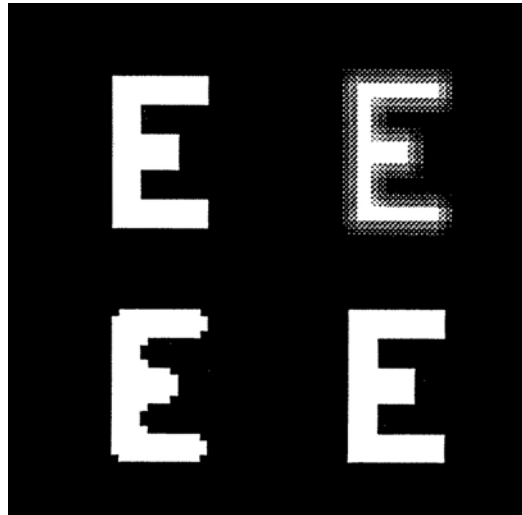
Figure 7.2: E (upper left) and after 3 \times 3 filtering by mean (upper right), 3 \times 3 median (lower left), and 3 \times 3 median with clipped corners (lower right)
